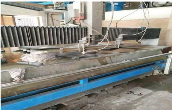
Fig2: Water jet Machine
