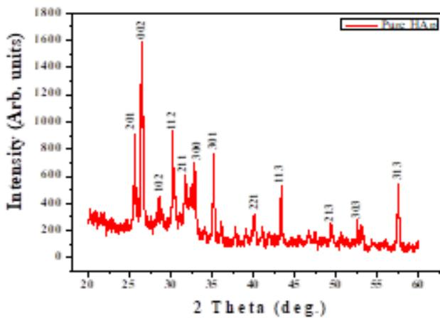
**Fig.1:** XRD pattern of pure HAp thick films
