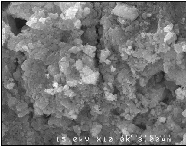
**Fig.3:** SEM pattern of pure HAp thick films
