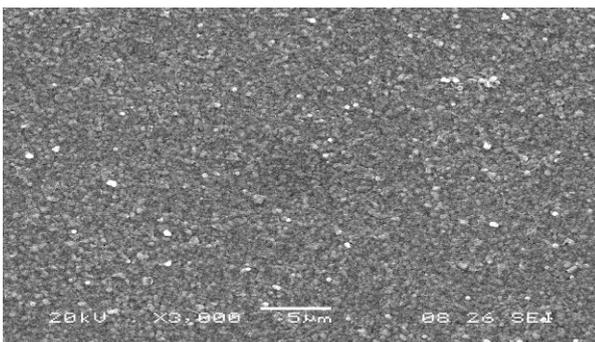
Fig : SEM image of CdS thin film
