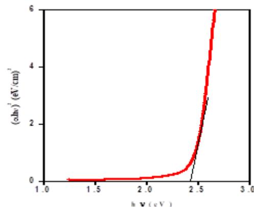
Fig 4. Optical absorption spectra of CdS thin film
