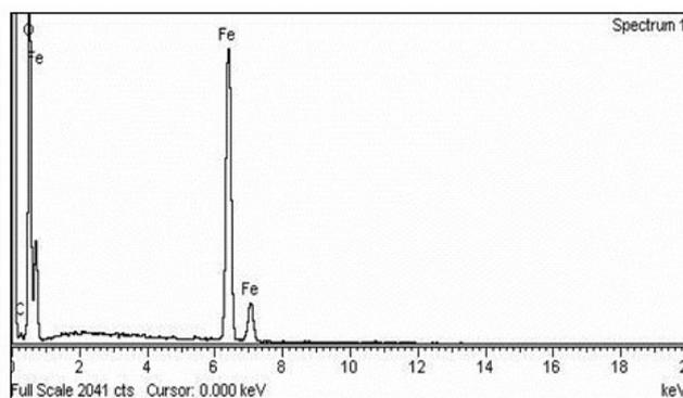
**Fig. 4:** EDS Spectra for Iron oxide Nanoparticles
