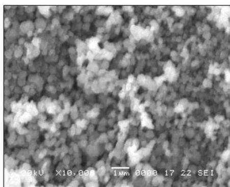
**Fig. 3:** SEM Image of Iron oxide Nanoparticle
