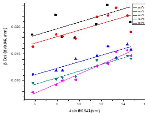
**Fig. 2:** W-H Plot for Iron oxide Nanoparticles
