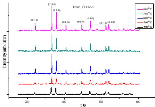
**Fig. 1:** XRD Spectra of Iron oxide Nanoparticles
