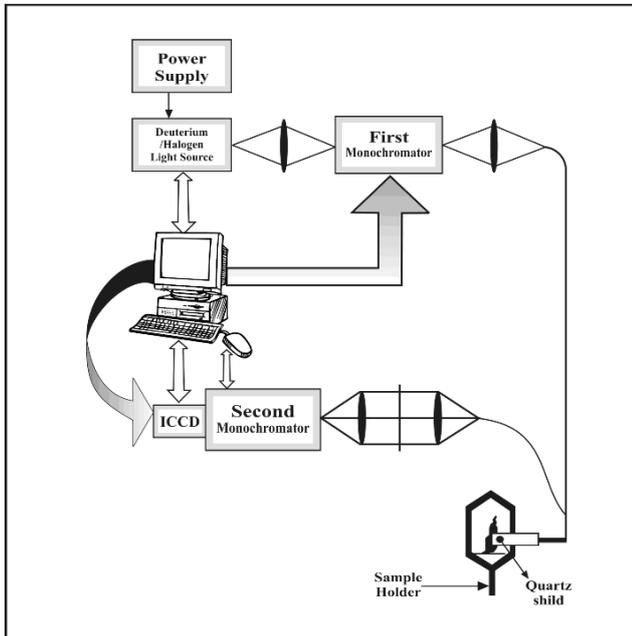
**Figure 1** Experimental arrangement for recording synchronous luminescence spectra of plants leaves. Commercial spectra physics fluorometer (SPEX, USA, Fluorolog -II) was used to record the synchronous luminescence spectra.
