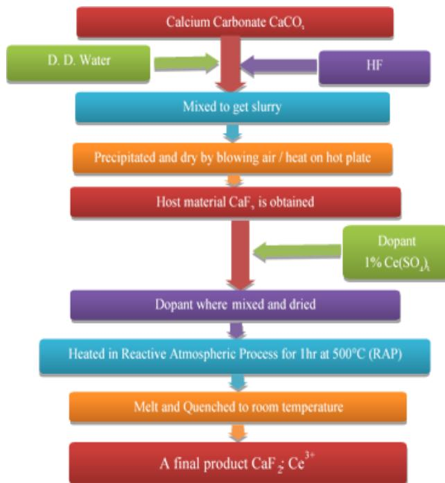
**Fig.1.** Flow chart of  $\text{CaF}_2$ :  $\text{Ce}^{3+}$  prepared via RAP.
