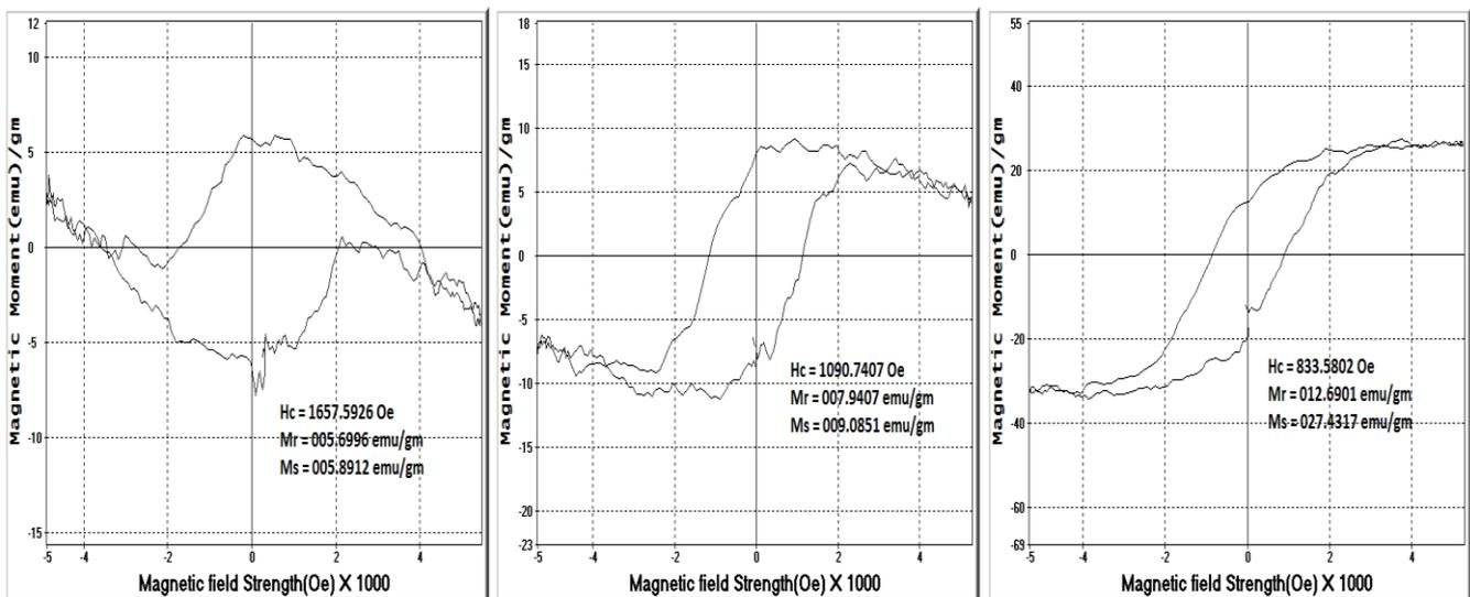
Figure 2: (a) VSM of  $\text{Pb}_{1.8}\text{Co}_{0.2}\text{Fe}_2\text{O}_4$  Fig3: (b) VSM of  $\text{Pb}_{1.6}\text{Co}_{0.4}\text{Fe}_2\text{O}_4$  (c) : VSM of  $\text{Pb}_{1.4}\text{Co}_{0.6}\text{Fe}_2\text{O}_4$
