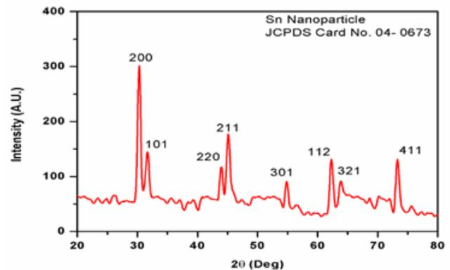
Fig 2. XRD spectra of synthesized Sn nanoparticles.
