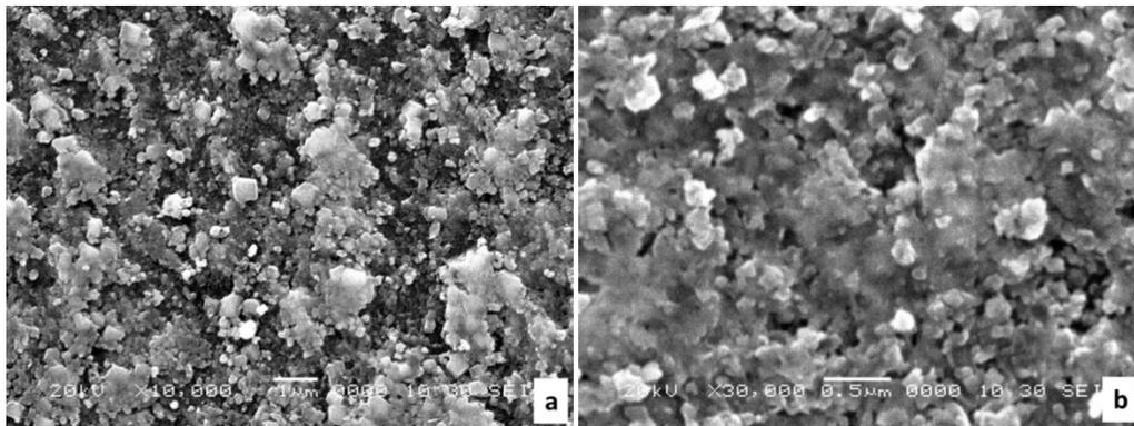
Fig 4: SEM images of electro-deposited Sn nanoparticles prepared at 3V potential
