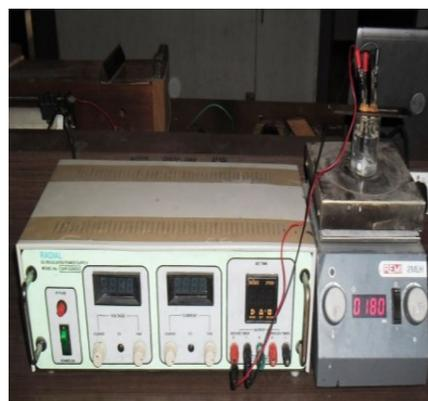
Fig 1. Electro-deposition Setup in the laboratory
