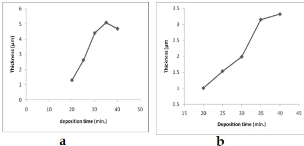
**Figure 2(a):** Change of Thickness with different deposition time on SS substrates**(b):** Variation of Thickness with deposition time on FTO coated glass substrates
