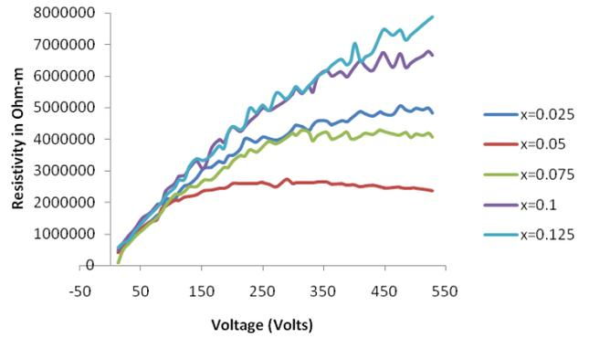
Fig.4: Graph of dc Resistivity with Voltage at  $200^\circ C$
