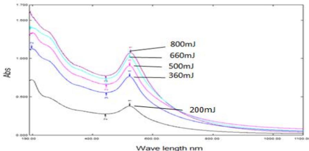
**Figure 1-** Absorption spectra of Au NPs.
