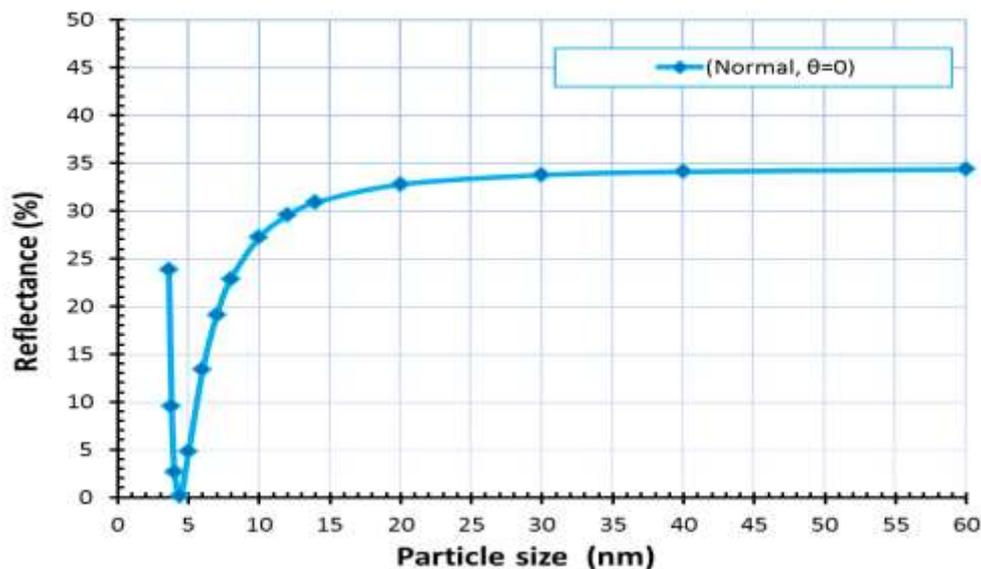
**Figure 1-** reflective design (Air/Nano Ge/(Si/Si) as a function of the particle size of the coating material, for the vertical fall, at the length of the design ( $\lambda_0 = 550$  nm), ( $L = 0.25 \lambda_0$ ).
