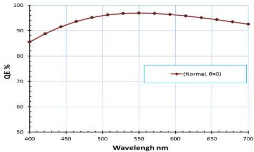
**Figure 4-** Quantitative Efficiency as a Function of the design Wavelength (Air/Nano Ge/si/si) at the Angle of ( $\theta_0 = 0^\circ$ )  $P_s = 4.4$  nm,  $L = 0.25\lambda_0$ ,  $\lambda_0 = 550$  nm.
