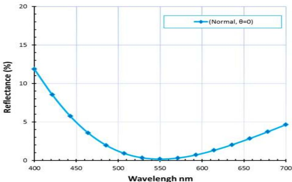
**Figure 3-** reflectivity as a function of the design wavelength (Air/Nano Ge/si/si) at the angle of ( $\theta_0 = 0^\circ$ )  $P_s = 4.4$  nm,  $L = 0.25\lambda_0$ ,  $\lambda_0 = 550 \text{ nm}$ .
