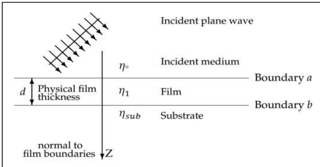
The Figure Shows a Low-level Wave on a Thin Film [18]
