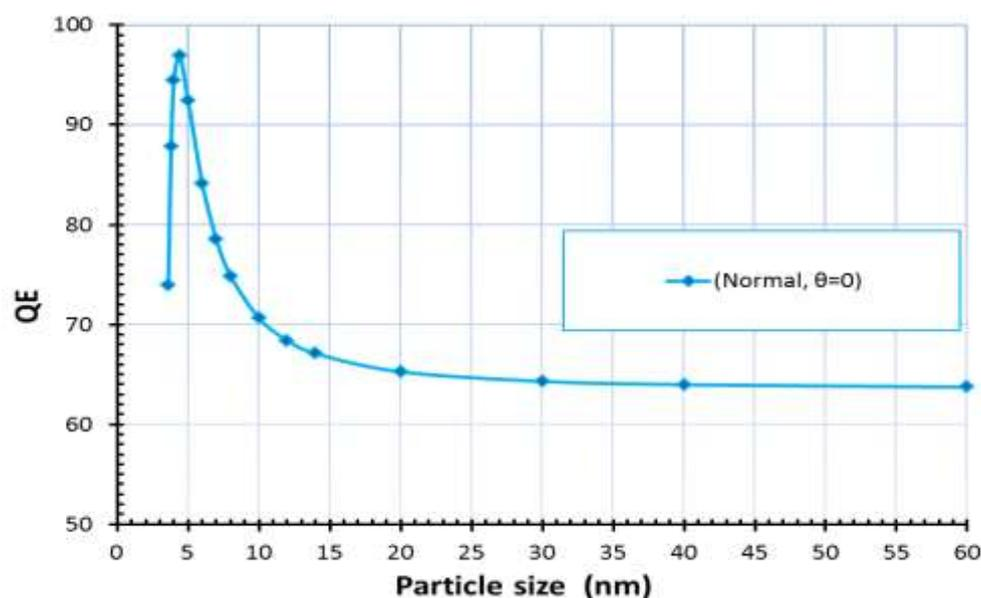
**Figure 2-** Quantity efficiency design (Air/Nano Ge/(Si/Si) as a function of the particle size of the coating material, for the vertical fall state, at the length of the design ( $\lambda_0 = 550$  nm), ( $L = 0.25 \lambda_0$ ).
