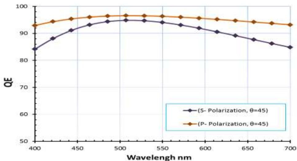
**Figure 6-** Quantitative Efficiency as a Function of the Wavelength for design (Air/Nano Ge/si/si) at the Angle of ( $\theta_0 = 45^\circ$ ),  $P_s = 4.4$  nm,  $L = 0.25\lambda_0$ ,  $\lambda_0 = 550$  nm.
