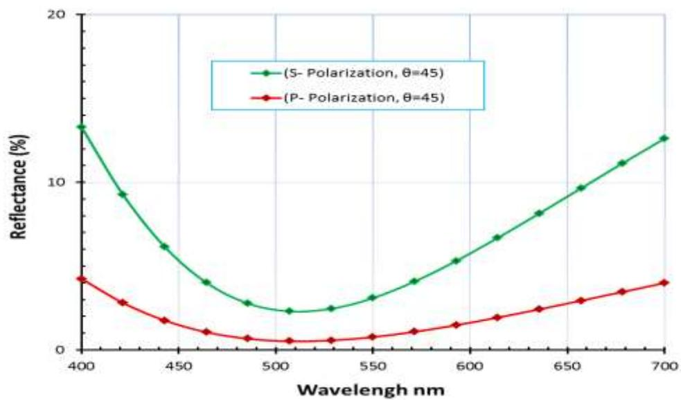
**Figure 5-** Reflective Wavelength as a Function for Design (Air/Nano Ge/(Si/Si) at the Angle of ( $\theta_0 = 45^\circ$ )  $P_s = 4.4$  nm,  $L = 0.25\lambda_0$ ,  $\lambda_0 = 550$  nm.
