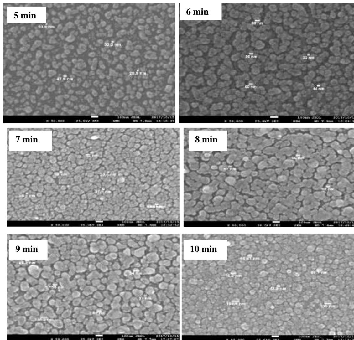
**Figure 3-**Shows the SEM image with magnification force = 50 kx of AgNP which had been prepared from 5 to 10 minutes as a reduction period.
