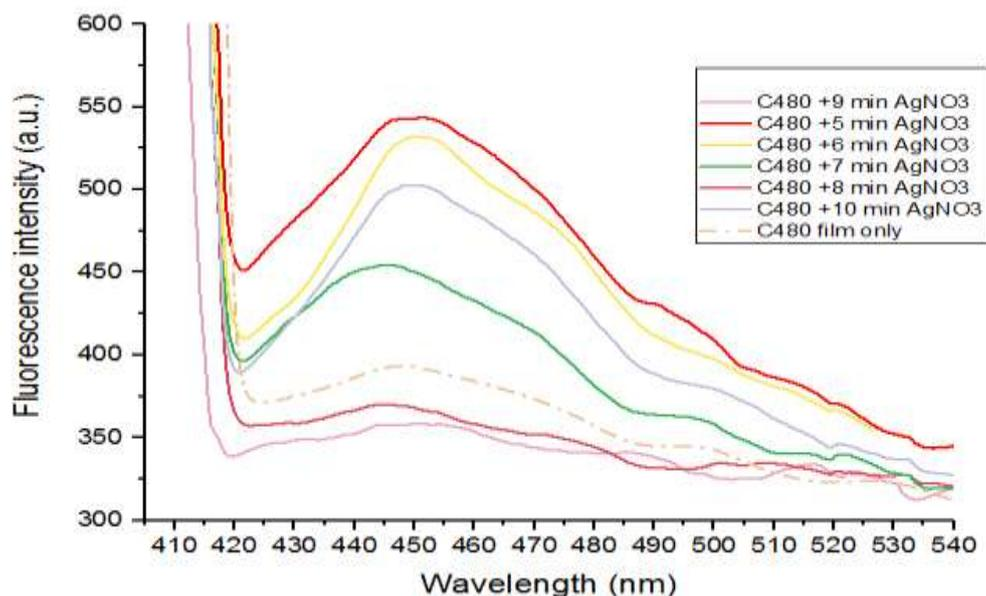
**Figure 7**-metal enhance fluorescence of AgNP-PVA -C480 sandwich (different reduction period).
