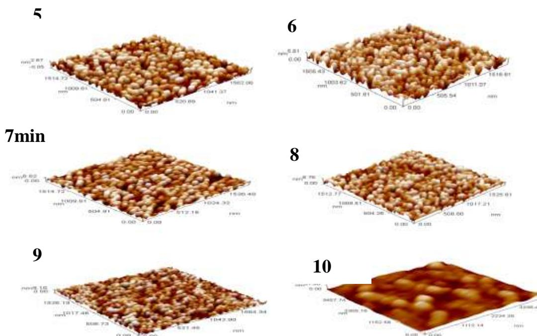
**Figure 2-** shows 3D images the AFM result for AgNP which is prepared by using different reduction period
