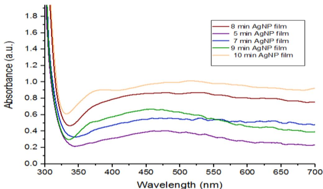
**Figure 4-**The absorbance spectra for silver nanoparticle film which is prepared by hot chemical reduction method as a function to reduction period.
