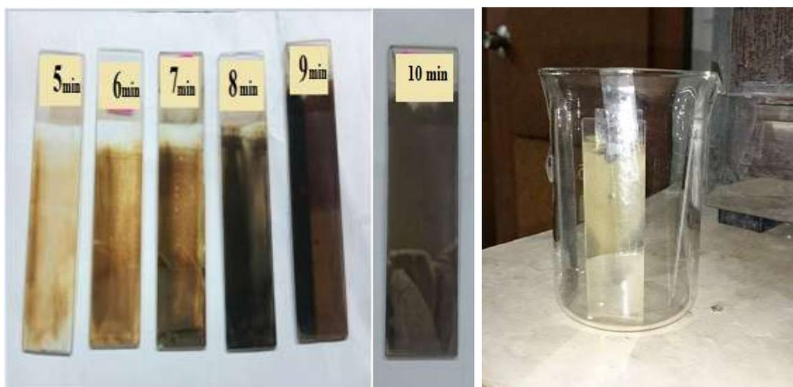
**Figure 1-**AgNP deposited on glass microscope slides by putting the slide in the hot rotation Ag NP solution at different reduction period
