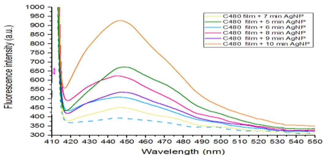
**Figure 5-**metal enhance fluorescence of AgNP-silica -C480 sandwich (different reduction period).
