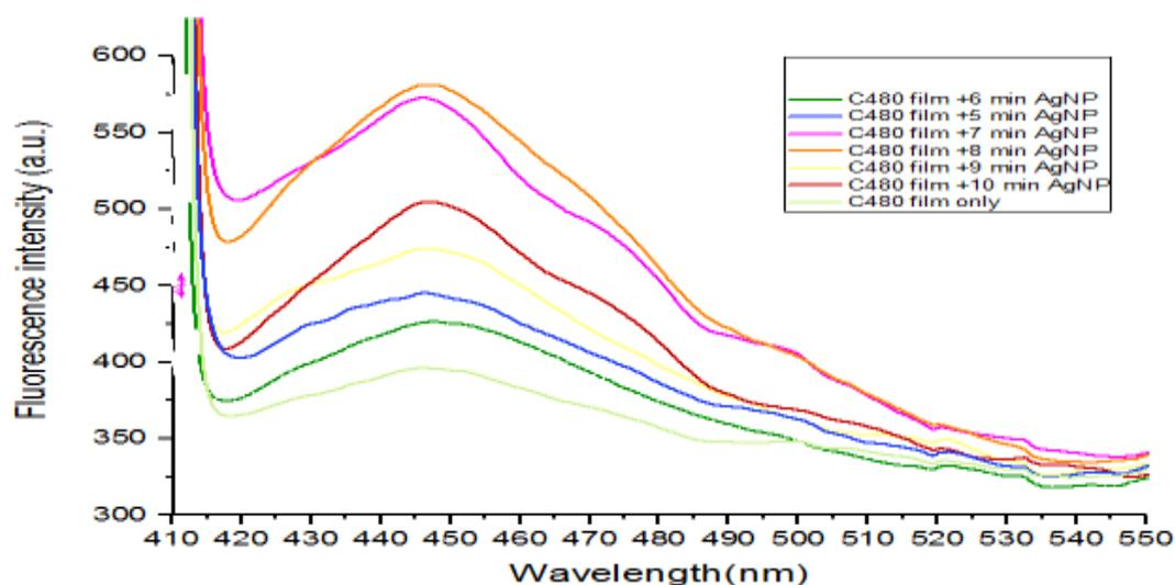
**Figure 6-**metal enhance fluorescence of AgNP-PMMA -C480 sandwich (different reduction period) Enhancement factor 1.47.
