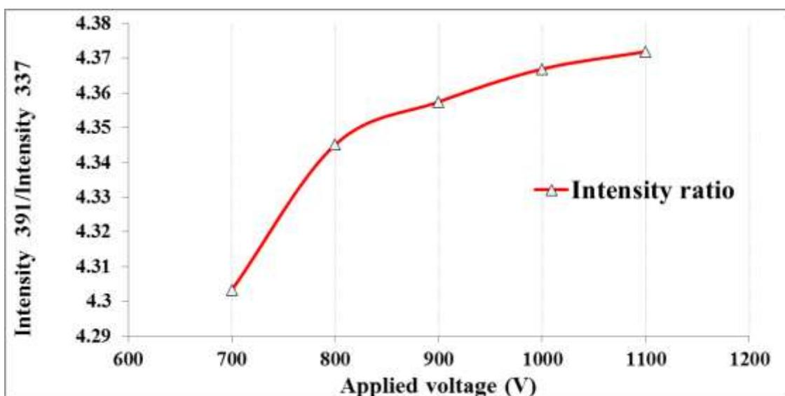
**Figure 10-**Variation intensity ratio between the two lines ( $I_{391.4} : I_{336.6}$ ) with applied voltage using Aluminum target.
