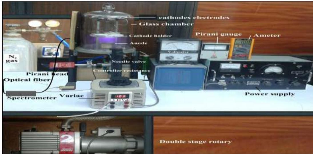
**Figure 3-**The image of DC discharge system with.
