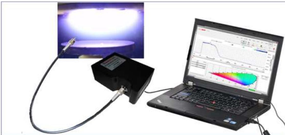
**Figure 4-**The image of spectroscopy measurement setup
