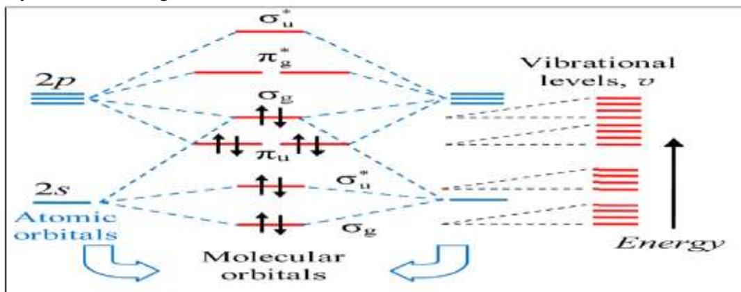
**Figure 2-** The molecules of nitrogen perform vibrations as fashioned by the particular electron occupancy of bonding versus anti-bonding (\*) molecular orbitals [7]
