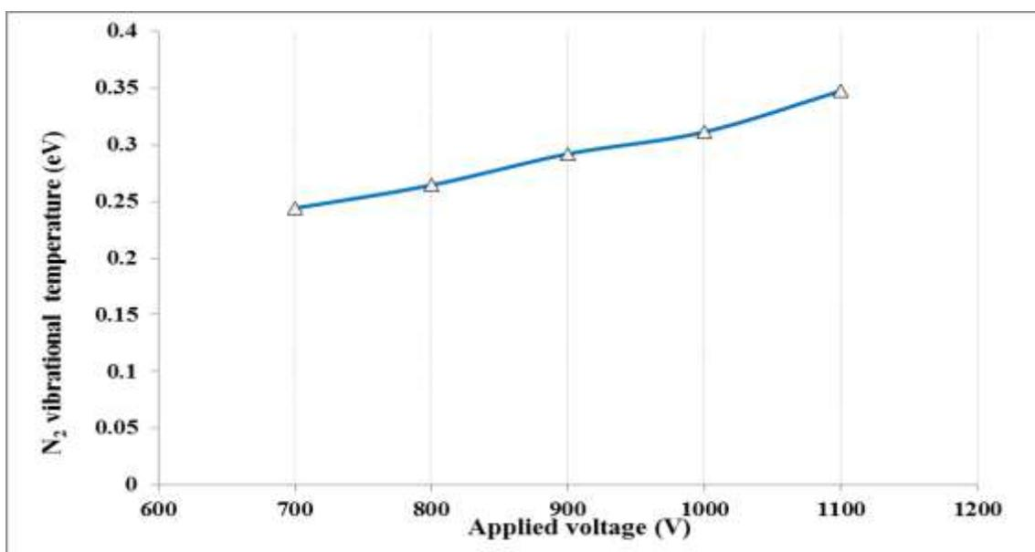
**Figure 11-** variation of vibrational temperature with applied voltage using Al target.
