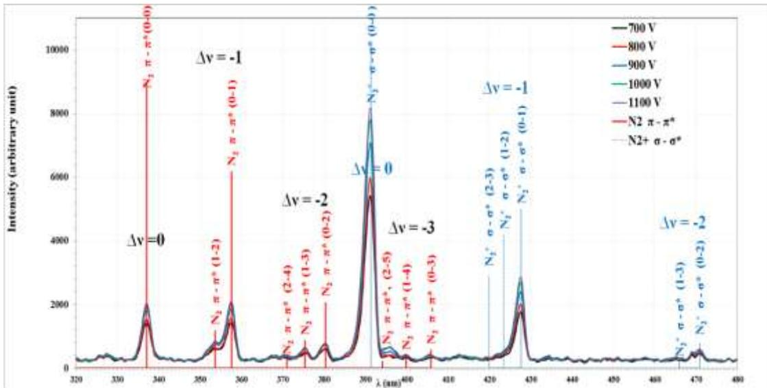
Figure 8-Matching the emission patterns, for different applied voltage using Al target, with N<sub>2</sub> molecular lines.
