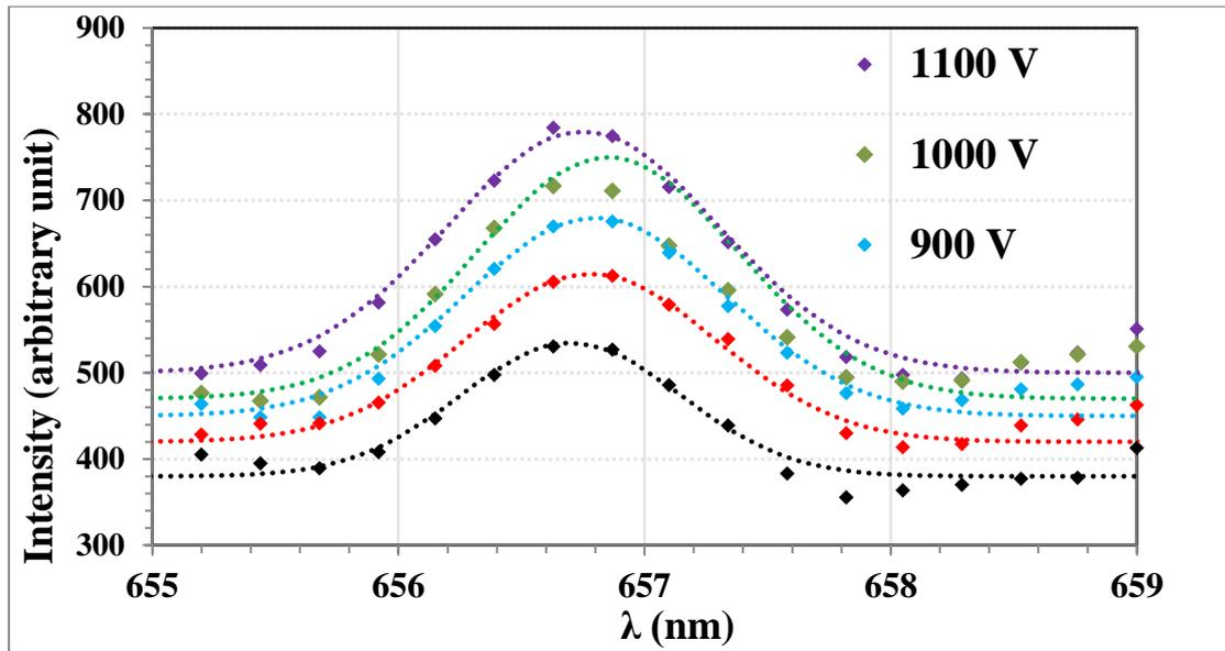
**Figure 6-** H $\alpha$  (656.28 nm) peaks broadening and Gaussian fitting at different applied voltage using Al target in nitrogen gas.
