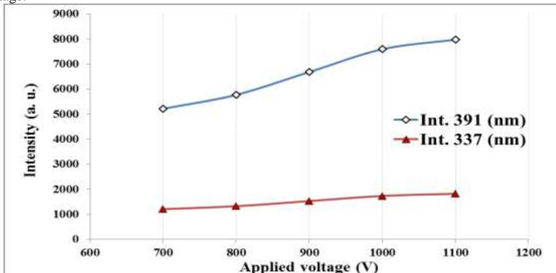
Figure 9-Variation of line intensities for pure electronic transition with applied voltage using Aluminum target.
