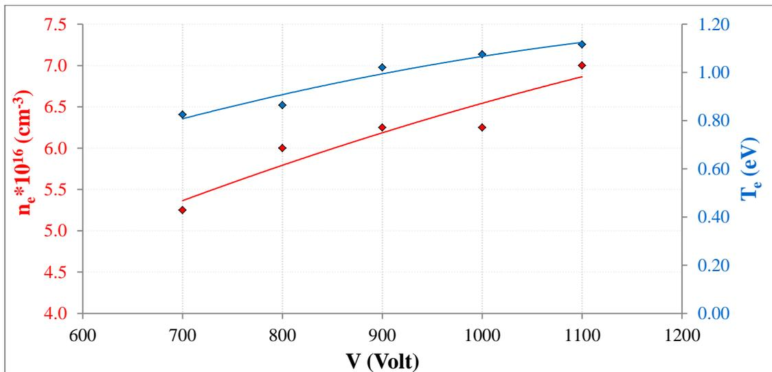
**Figure 7-** The variation of  $T_e$  and  $n_e$  for DC plasma in  $N_2$  with different applied voltage using Al target at constant working pressure (0.2 mbar) with 3 cm inter electrode distance.
