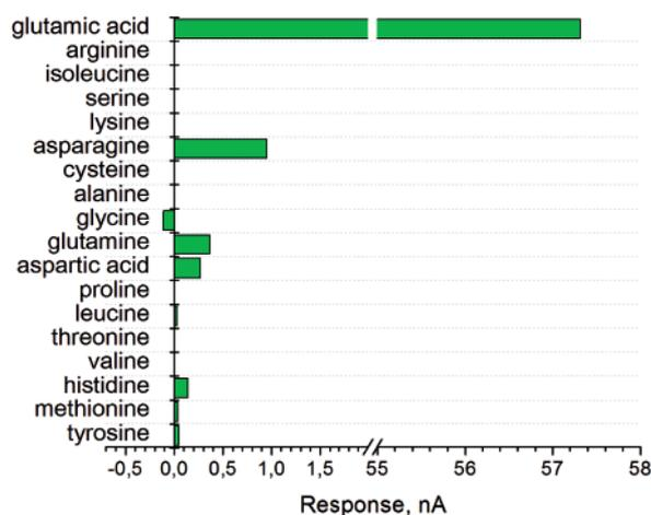
**Fig. 2. Biosensor responses to various amino acids:** concentration of each amino acid was 1 mM. Measurements were carried out in 25 mM HEPES buffer, pH 7.4, at a constant potential of +0.6 V vs Ag/AgCl reference electrode
