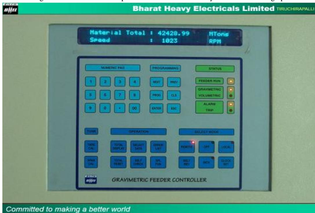
Figure 3: The HMI panel of BHEL GFC system
