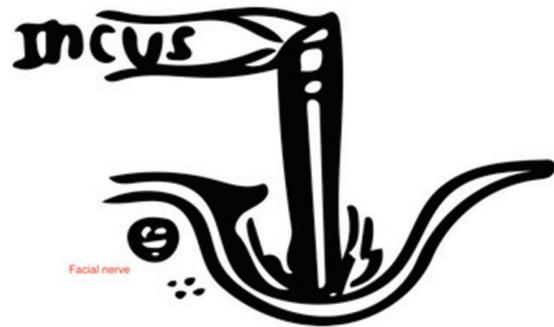
Fig 3. Proper position of tailor-made polyethylene strut prosthesis connected between lenticular process of incus and oval window
