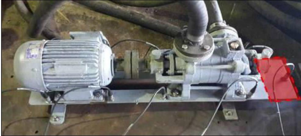
**Figure 2.** Electric Motor Driven Pump Set-up
