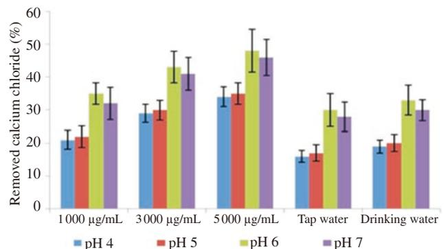
**Figure 4.** Removal of calcium chloride from ground water and pure solutions of higher concentrations at different pH conditions by *A. niger*.
