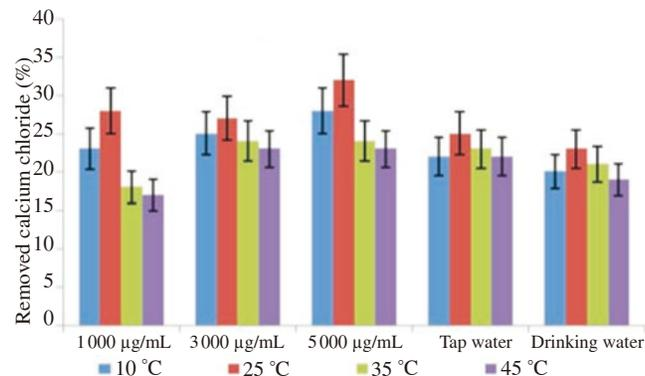
**Figure 7.** Removal of calcium chloride from ground water and pure solutions of higher concentrations at different temperature conditions by *A. niger*.
