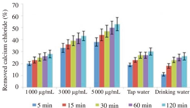
**Figure 1.** Removal of calcium chloride from ground water and pure solutions of higher concentrations by *A. niger*.
