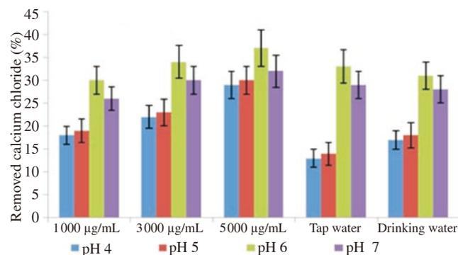
**Figure 5.** Removal of calcium chloride from ground water and pure solutions of higher concentrations at different pH conditions by *N. crassa*.
