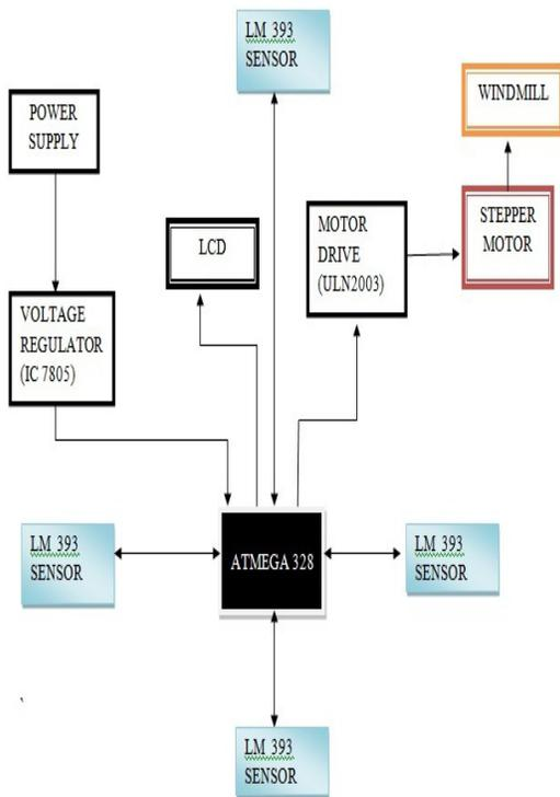
**Fig 1. Block Diagram of Wind Turbine using Micro Controller**
