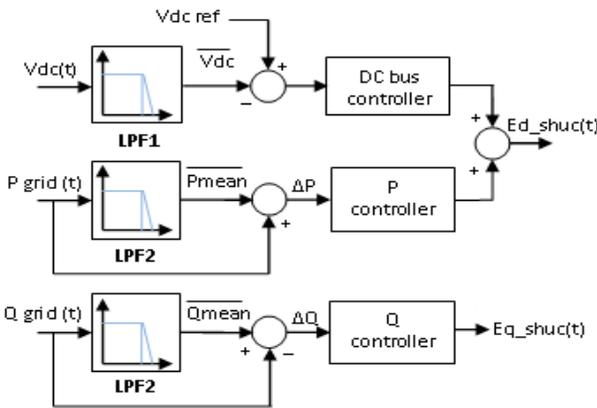
Figure 6. Shunt compensator controller
