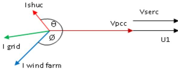
Figure 3. Phasor diagram of UPQC
