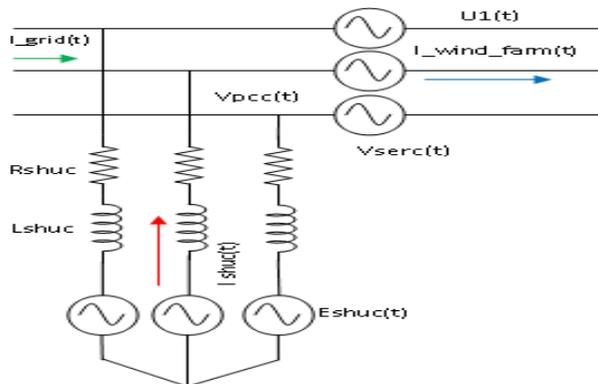
Figure 4. Power stage compensator model. AC side
