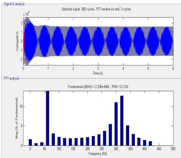
Fig.9. Result Of power system without UPQC
