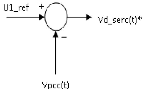
Figure 5. Series compensator controller
