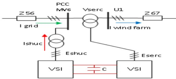
Fig (2): Block diagram of UPQC
