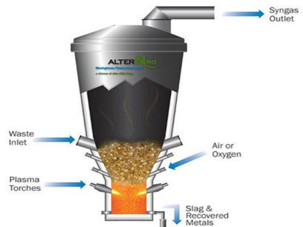
Fig. 3 Plasma gasification process
