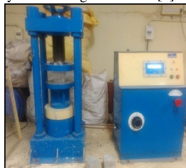
Figure 1: Compressive strength testing by UTM of capacity 40 tonnes
