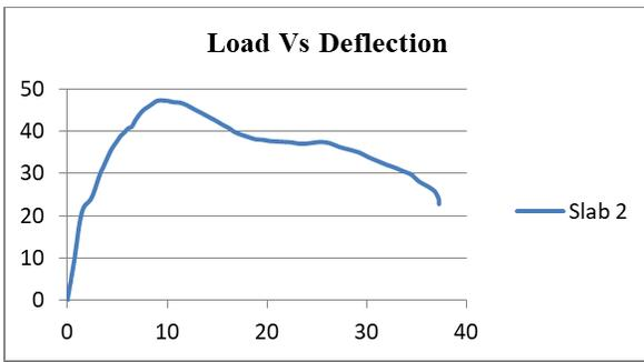
Fig. 8 Load vs. deflection graph for SB- 2
