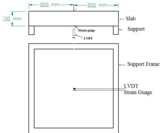
Fig. 4 Schematic diagram of test set up
