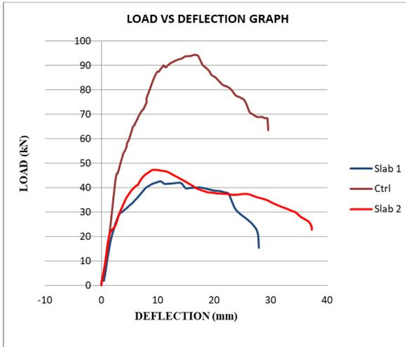
Fig. 9 Load vs. deflection comparison graph
