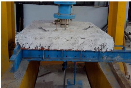
Fig. 5 Hollow core slab test set up
