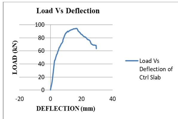
Fig. 6 Load vs. deflection graph for SB- C
