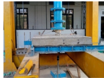
Fig. 6 Slab with topping test setup
