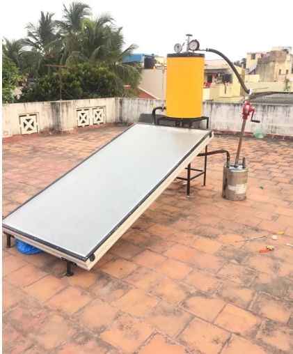
Figure 1.1 Complete structure of the desalination plant
