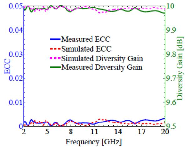
Figure 10 Measured and Simulated ECC and Diversity Gain
