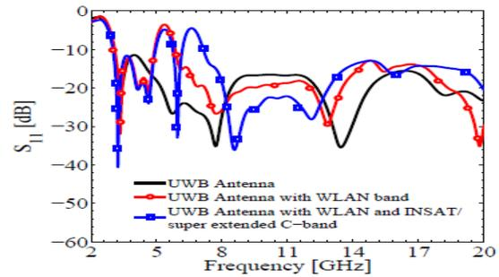
Figure3.2 Simulated  $S_{11}$  against Frequency for the Various configurations of Radiator
