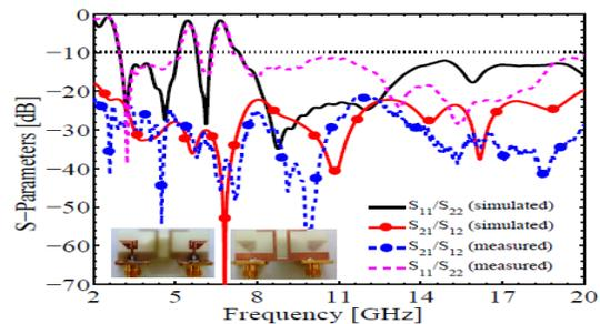
Figure 8 Simulated and Measured S-parameters Results for the UWB MIMO-Diversity Antenna
