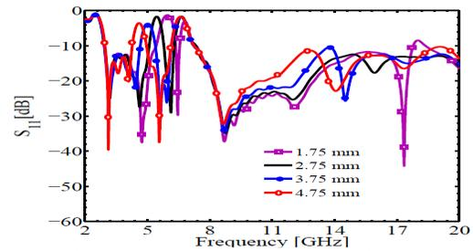
Figure 6. Simulated S-parameters against Frequency for the Various values of  $L_{p3}$
