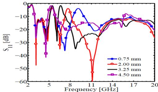
Figure 7 Simulated S-parameters against Frequency for the Various values of  $L_{p4}$
