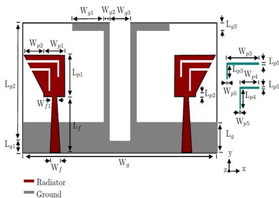
Figure.1 Geometry of the Proposed MIMO/Diversity Antenna
