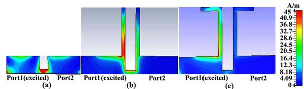
Figure 4 Current Distributions at Various Geometry of the Ground Plane
