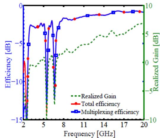
Figure 11 Efficiency and Realized Gain for the Proposed MIMO Antenna For uniform 3D-angular power spectrum and high signal-to-noise ratio(SNR),  $\eta_{MUX}$  is given by [22]
