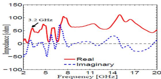
figure 3.1 simulated input impedance versus freq
