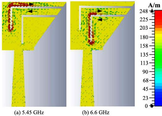
Figure 5: Current Distributions of the Proposed MIMO Antenna at (a) 5.45 GHz (b) 6.6 GHz
