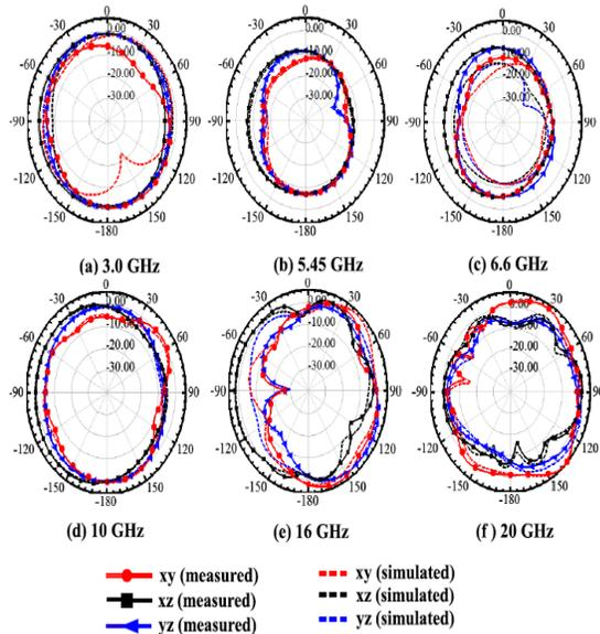
Figure 9 Radiation Pattern for the Proposed MIMO Antenna at (a) 3.0 GHz (b) 5.45 GHz (c) 6.6GHz (d) 10 GHz (e) 16 GHz and (f) 20 GHz
