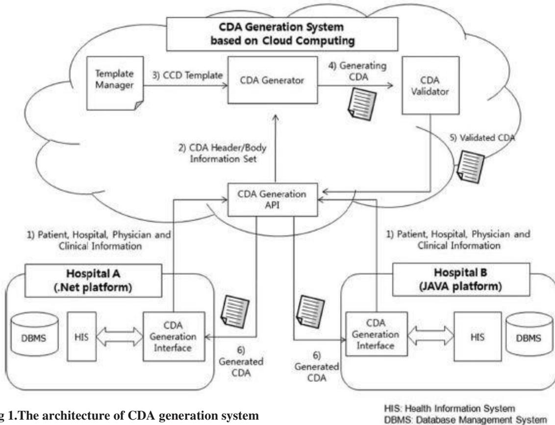
Fig 1. The architecture of CDA generation system
