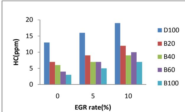
Fig -7: Variation of hydrocarbon with EGR.
