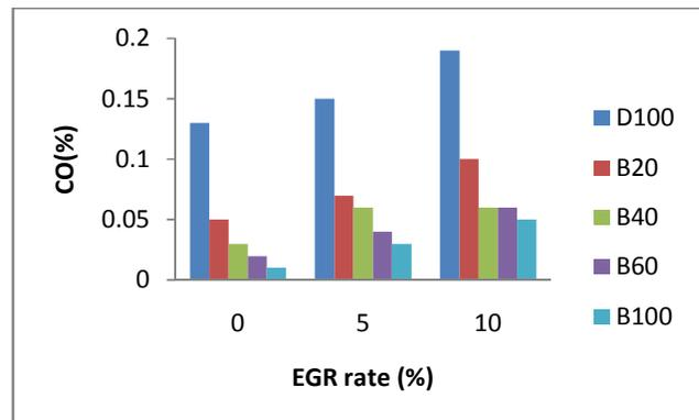
Fig -6: Variation of carbon monoxide with EGR. Fig.6 shows the variation of carbon monoxide emission with EGR at full load for diesel and blends of corn oil biodiesel. The CO emission depends upon the strength of the mixture, availability of oxygen and viscosity of
