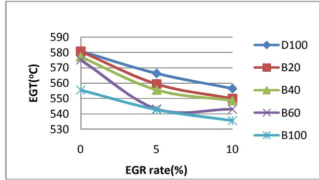
Fig -5: Variation of exhaust gas temperature with EGR.
