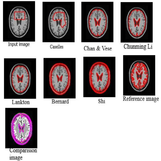
Fig 2: Segmented images obtained from various level set algorithms.
