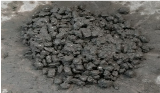
Fig 4.3 Mixture of no-fines aggregate
