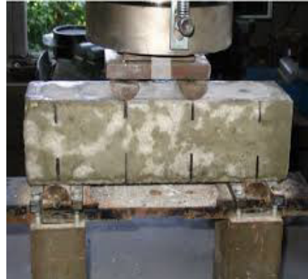
Fig 4.9: Concrete Beam Specimen for Flexural Strength Test
