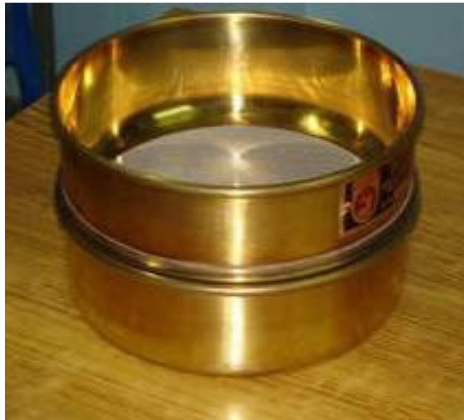
Fig 4.2.2.1.2 Sieve used for find fineness of cement
