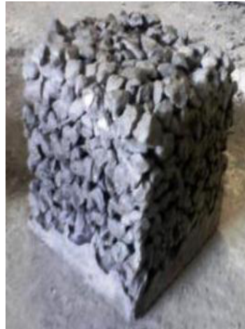
No fines concrete cube
