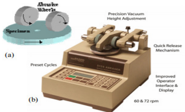
Figure: 1.1. Rotary Platform Abraders: (a) test principle and (b) test setup
