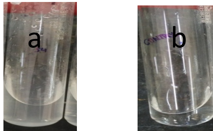
Figure 4: a) Growth in MSM supplemented with 1% Toluene b) Control tube with no growth
