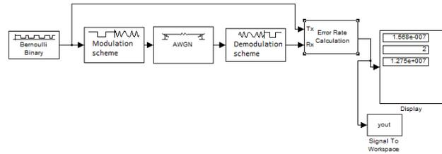
Fig.3. Digital Communication System model created using Simulink
