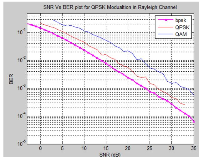
Fig. 4 BER Performance of BPSK, QPSK & QAM using simulink model
