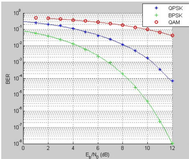
Fig. 2 BER Performance of BPSK, QPSK & QAM in Rayleigh channel using MATLAB code
