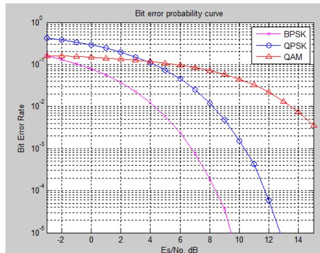
Fig. 1 BER Performance of BPSK, QPSK & QAM in AWGN channel using MATLAB code
