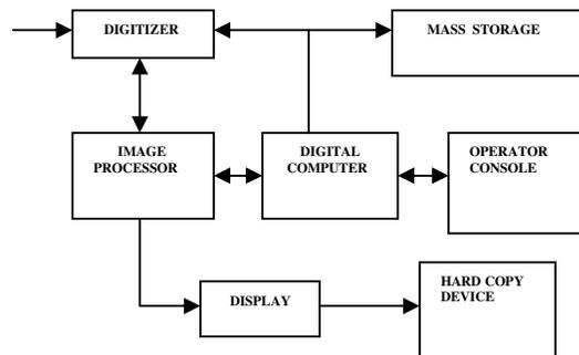
Fig. 1 Image Processing System
