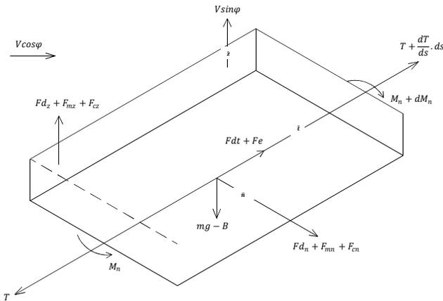
Figure 3: Forces and moments acting on a cable element
