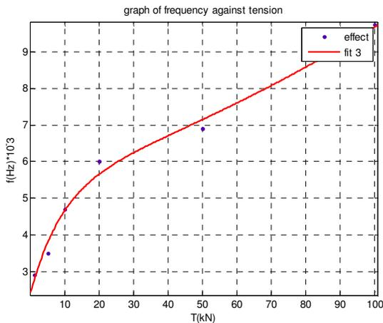
Figure 11: Graph of frequency against tension in transverse direction based on 30kg/m
