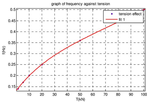
Figure 10: Graph of frequency against tension in transverse direction
