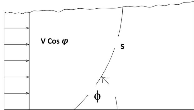
Figure 1: Schematic of an umbilical cable under-sea
