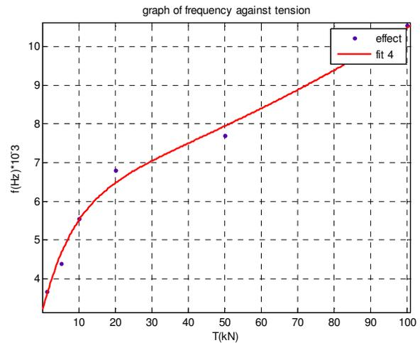
Figure 12: Graph of frequency against tension in transverse direction based on 60kg/m
