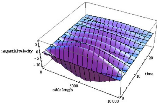
**Figure 7: Graph of tangential velocity against time and length**
