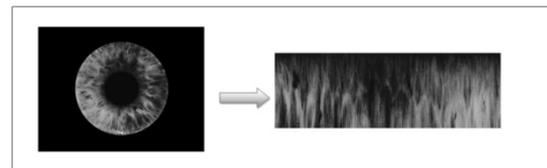
Fig. 2: Segment iris into polar coordinates
