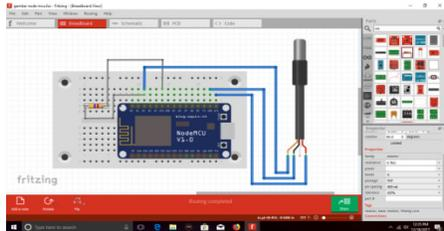
Figure 4.8 Schematic Node Mcu Esp8266 With Ds18b20 Sensor
