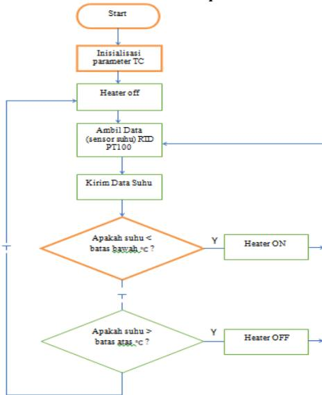
Figure 4.4 Diagram of On-Off Method
