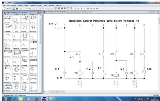
Figure 4.2 Results of Tool Control Circuits Temperature Monitor
