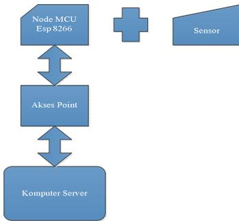
Figure 4.7 Tool Design Hard Block Diagram
