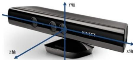
Fig.1 Kinect sensor
