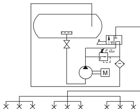
**Figure 1.** Schematic representation of sprayer installation components
