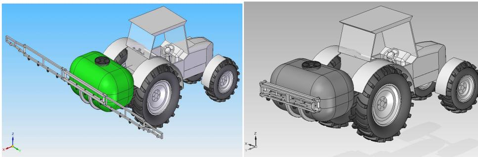
a) The working position for sprayer installation
