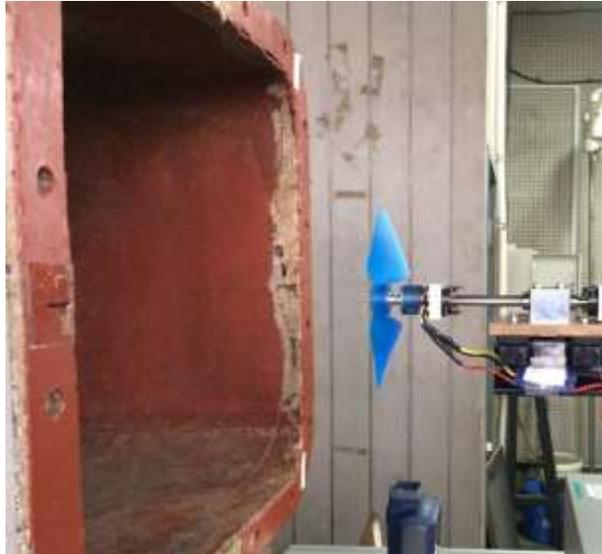
Figure 7: Propeller on Wind tunnel test stand
