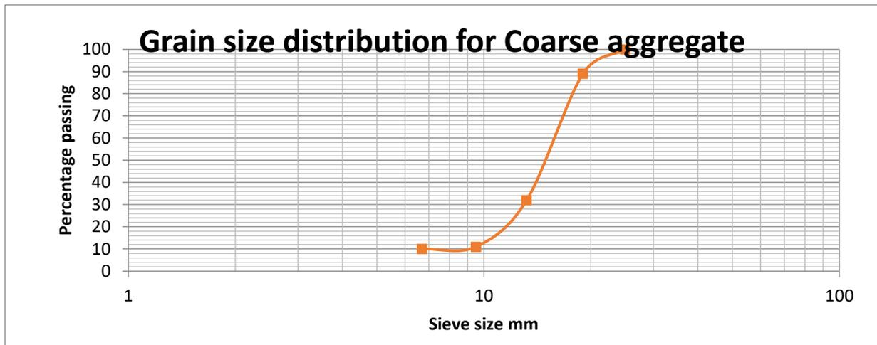
Figure 3: Percentage passing against sieve sizes (Coarse aggregate)
