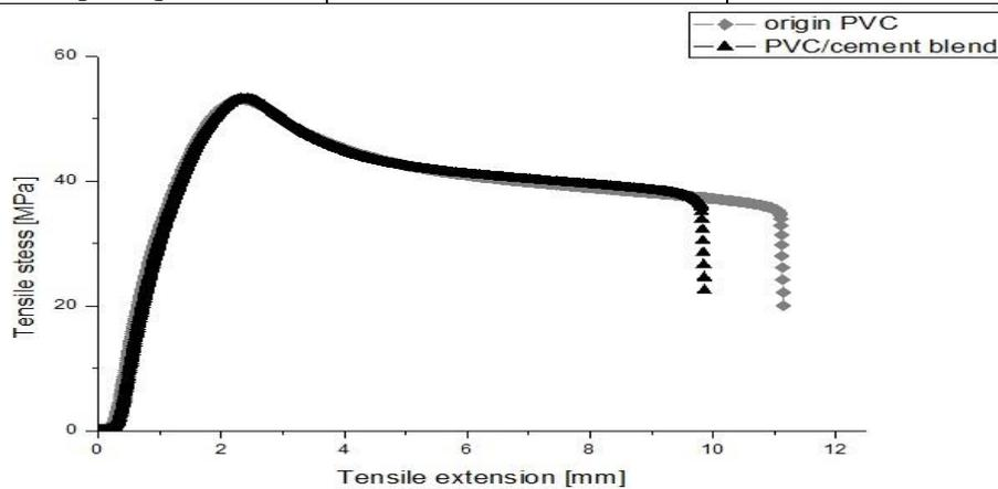
Figure 1: Original and blend tensile stress-strain curves
