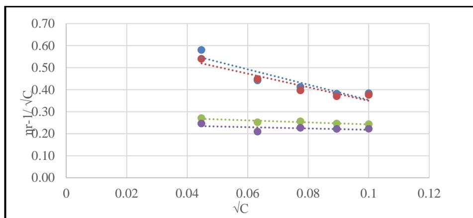
**FIGURE 2:** Plot of  $(\eta_r - 1)/c^{1/2}$  vs  $c^{1/2}$  of N-phenyl maleanilic acid and N-phenyl maleimide in aqueous dimethyl sulfoxide at 308.15 and 313.15 K.
