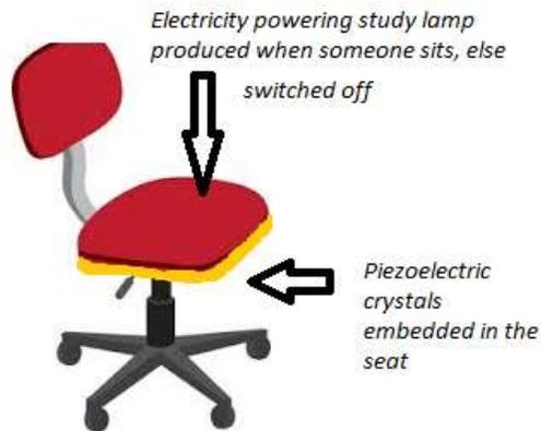
**Fig.4. Piezoelectricity powered study lamp**
