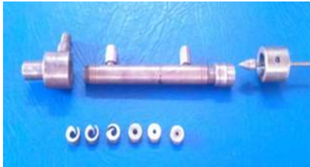
Fig. 2: Parts of Vortex Tube used for experiments
