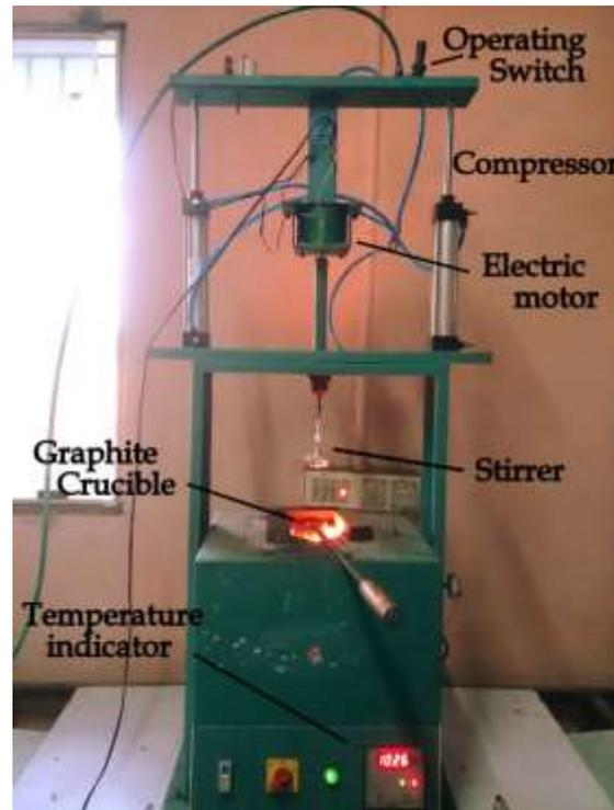
Figure 1. Stir Casting setup for fabrication of (Al8011/ B<sub>4</sub>C/ Red Mud)
