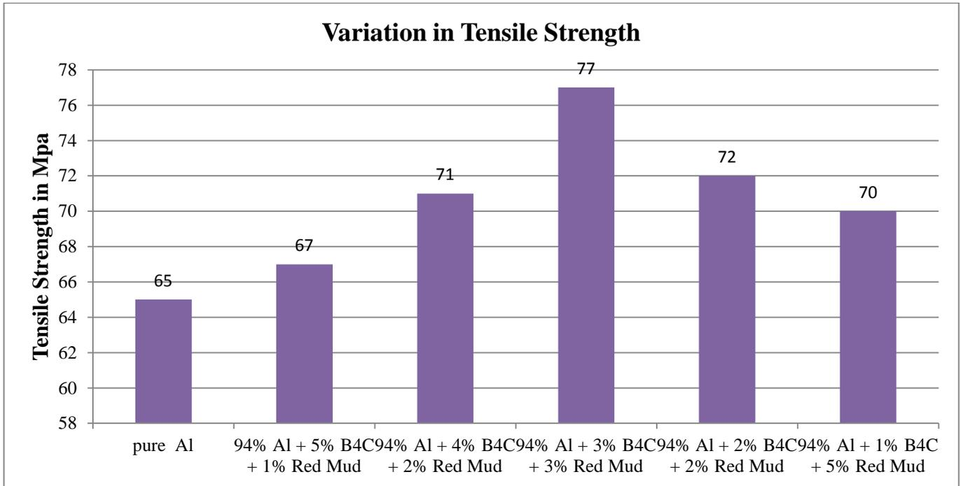
Fig.9 graph shows the variation in tensile strength from 5-1% of B<sub>4</sub>C and 1-5% Red mud composite
