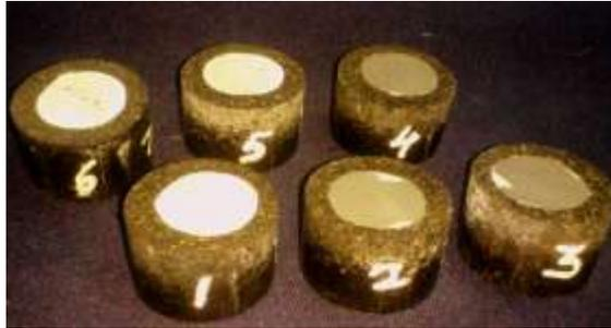
Figure 4. Prepared specimens for Vickers Hardness Test
