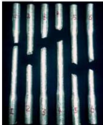
Figure 3. Specimens which undergone Tensile Test.
