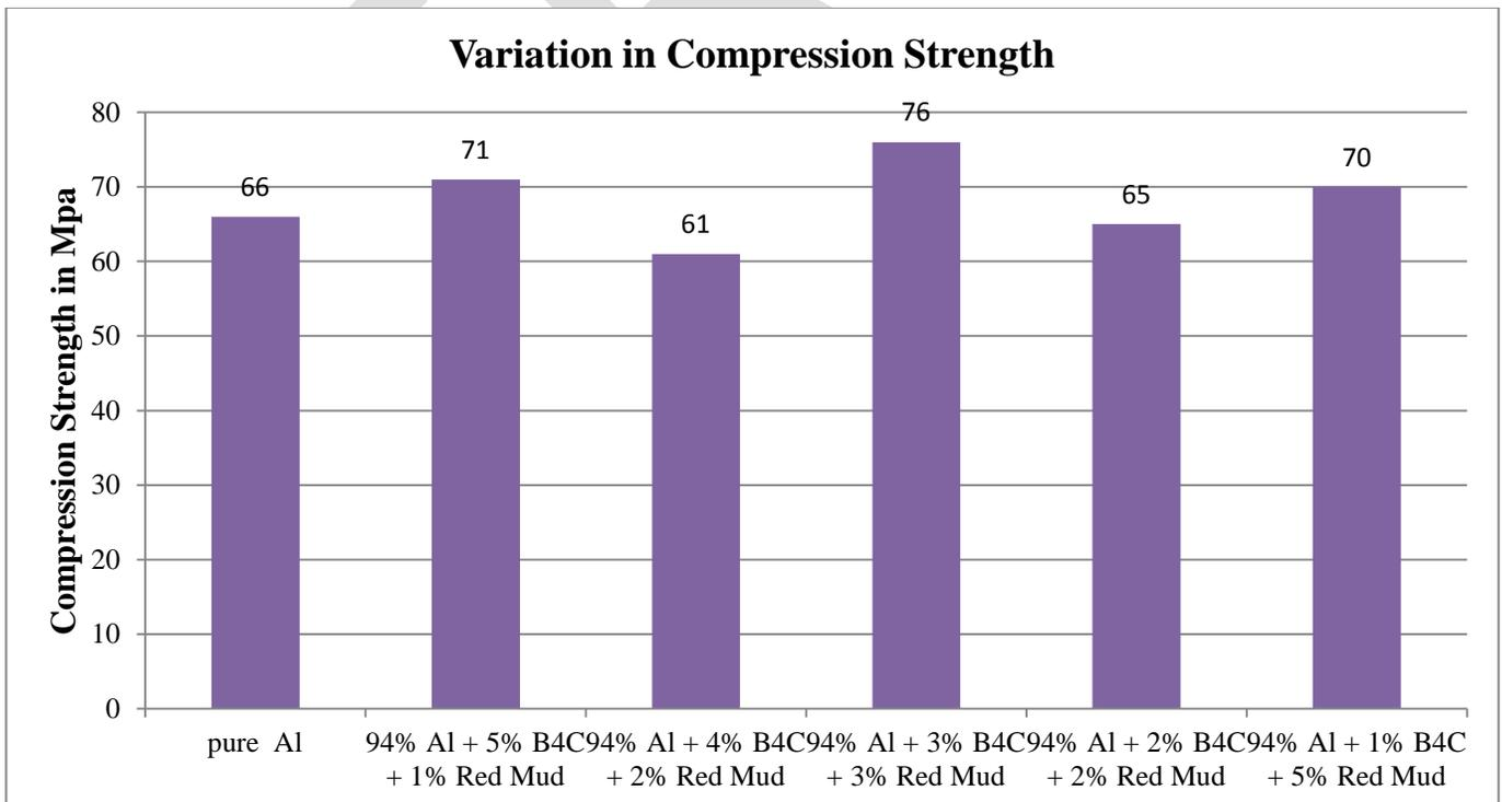
Fig.10 graph shows the variation in Compression strength from 5-1% of B<sub>4</sub>C and 1-5% Red mud composite
