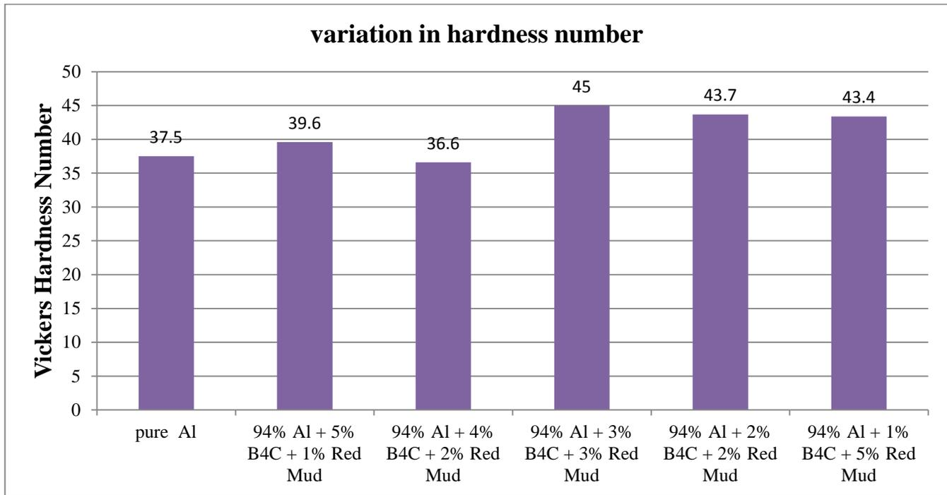
**Fig.11 graph shows the variation in Hardness Number from 5-1% of B<sub>4</sub>C and 1-5% Red mud composite**
