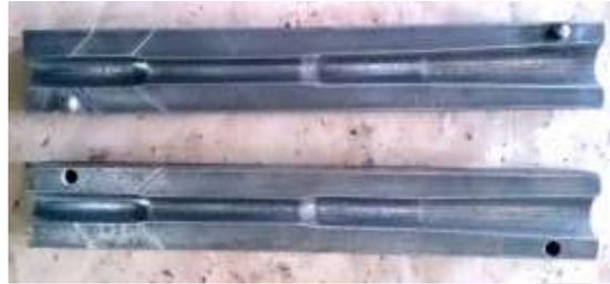
Figure 2. Die used for Stir Casting
