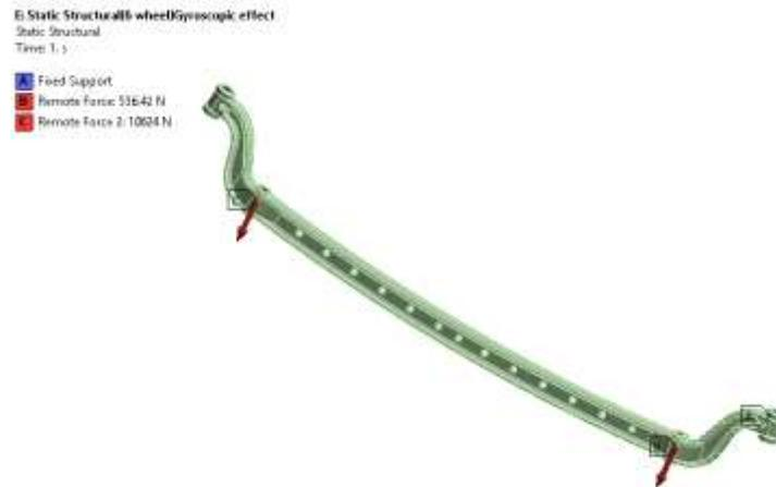
Figure.3. Boundary conditions due to gyroscopic effect
