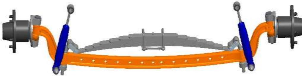
**Figure.1. Dead Front Axle Mechanism of Commercial Truck**
