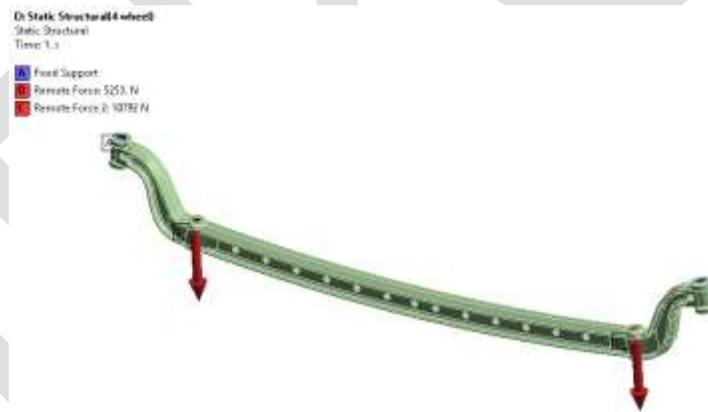
Figure.4. Boundary conditions due to gyroscopic effect
