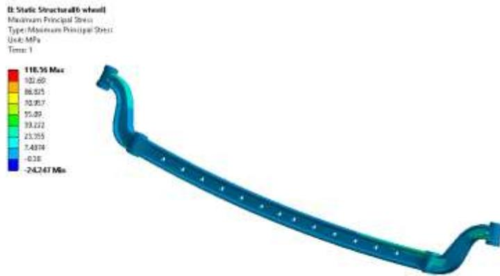
Figure.12. Maximum principal stress distribution for W<sub>1</sub> and W<sub>2</sub>
