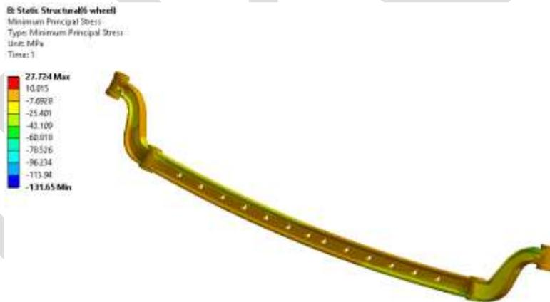
**Figure.13. Minimum Principle stress**
