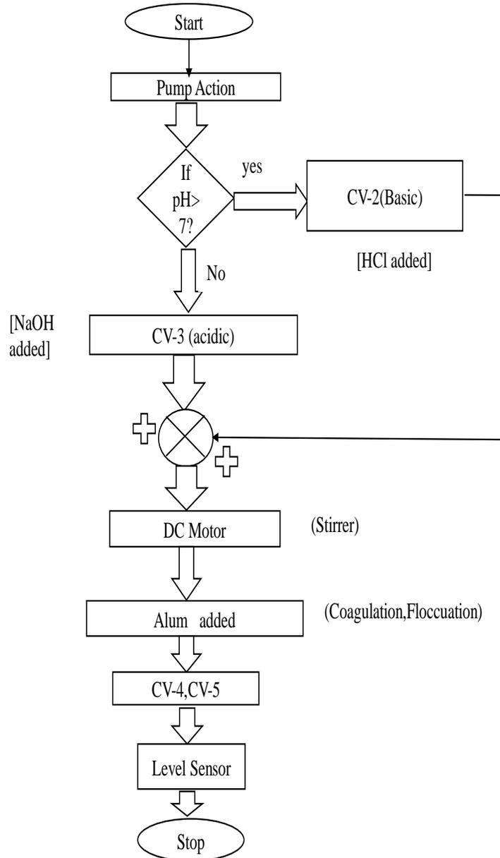
Fig.9 Flow Diagram of Process
