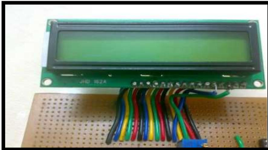
Fig.7 LCD Display
