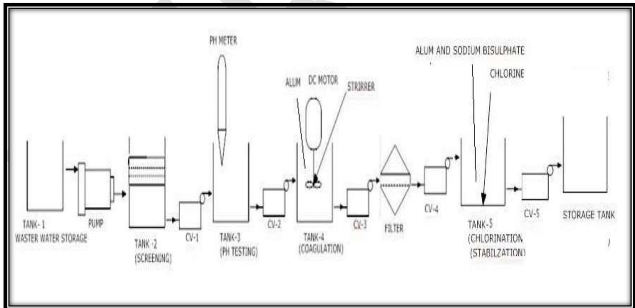
Fig.8 Process Diagram
