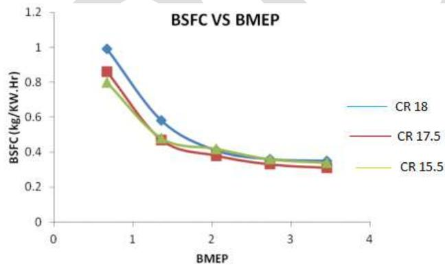
Chart.1: Brake specific consumption for variable compression ratio.
